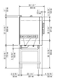
CWII Cold Water inlet 1 (cleaning) = Cold Water Inlet 2 (steam generator) CWI2
